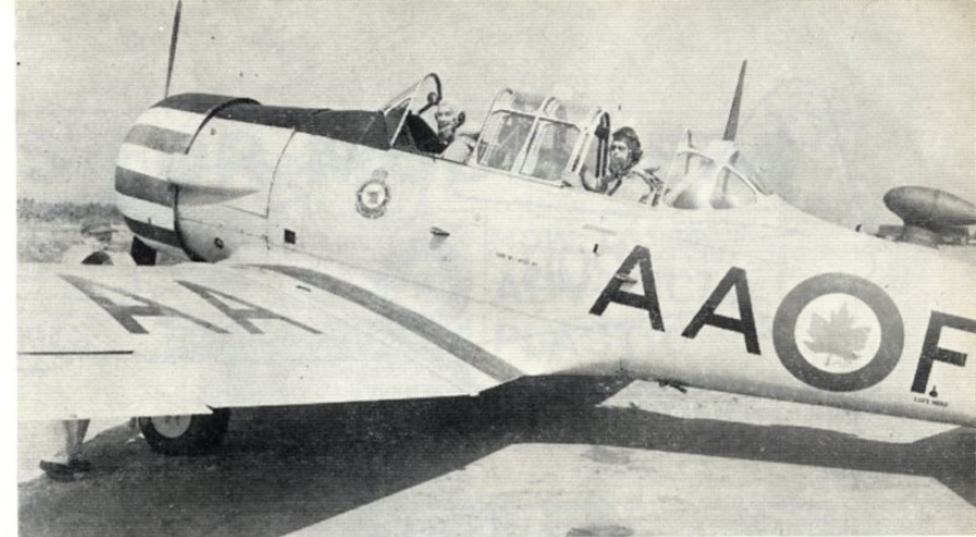
A Canadian-built Harvard IV belonging to No 400 Squadron RCAF—an auxiliary squadron stationed at Downsview, Toronto. Painted overall yellow, the cowling stripes are red and white. Codes and serials (in this case 3125 on the fin) are in black. The squadron crest, which consists of a Griffon's head in red surmounting two gold-coloured tomahawks, appears under the front cockpit (Doug Baker).
